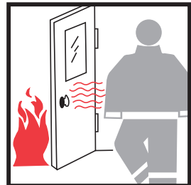
Radiant heat from hot surfaces and flames can cause burns.
