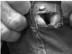
FIG. 2 Test fabric strength with thumbs
