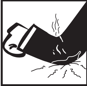
Compression against hot surfaces can cause burns
