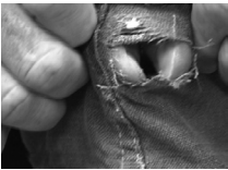
FIG. 2 Test fabric strength with thumbs
