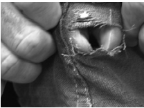
FIG. 2 Test fabric strength with thumbs
